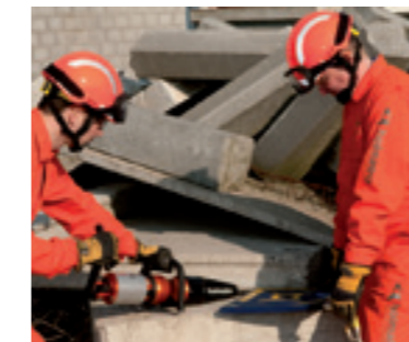
Power Wedge creates opening for lifting bag (see page 36)
